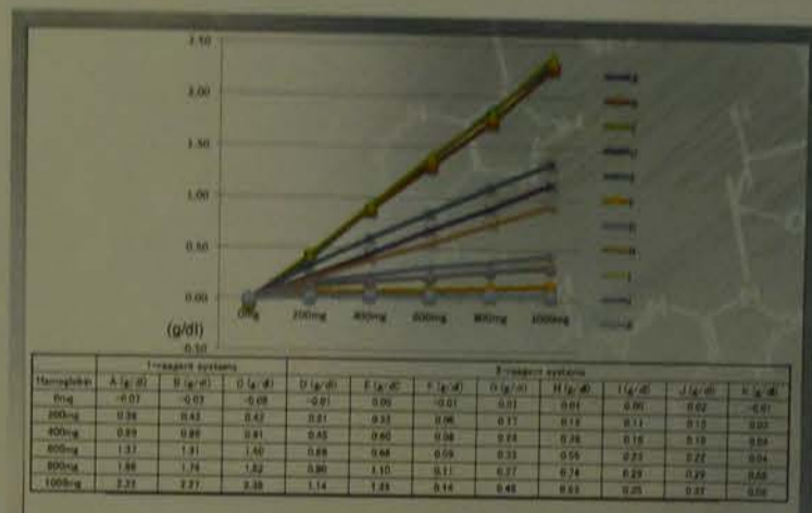
Fig. 2. Interferences of hemoglobin for the determination of serum total protein with eleven biuret assay.
